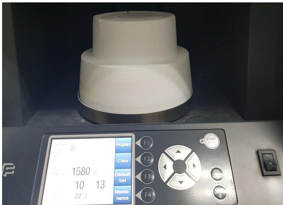
Run the program for 10 hours at up to 1580°C.
